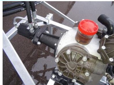
Hydraulic Drive of pump
