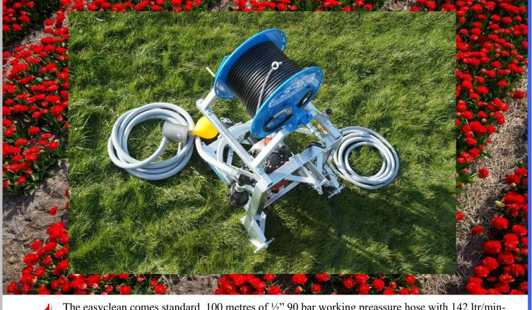
The easyclean comes standard 100 metres of ½" 90 bar working preassure hose with 142 ltr/min-50 bar piston diaphragm pump.
